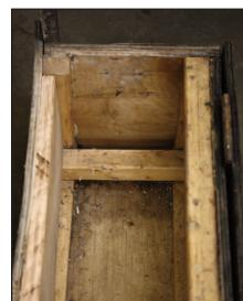
You should brace the box as in the picture since unsupported plywood warps. You need something to hold the paper off the bottom of the box and keep it dry; the bracing does that too. The roll of paper lies on the cross-braces and unrolls at the front so it has straight-up path to the crossbar.
